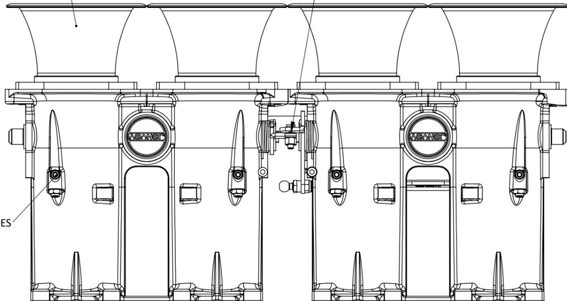
IDLE AIR ADJUSTMENT COMPLETED THROUGH BLEED SCREWS ON TOP OF THE THROTTLE BODIES
